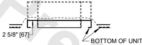
**TYPICAL BOTTOM INLET CONNECTION DETAIL**
