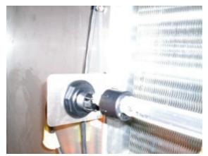
2. Plug the bulb into the four hole socket and make sure it is fully seated. Now slide the ring tight against the assembly and tighten the fitting. **Hand tighten only – never use a tool!** Failure to properly install the waterproof assembly can cause premature failure of the bulb.
