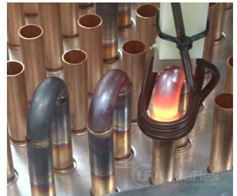
Figure 7: Induction Brazing of Copper Tubes
