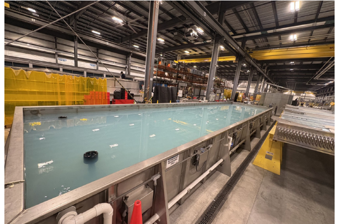
Figure 3: Test tank used for ASME pressure testing of coils.
