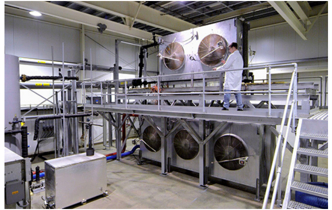
Figure 1: AHRI Evaporator test lab and technician.
