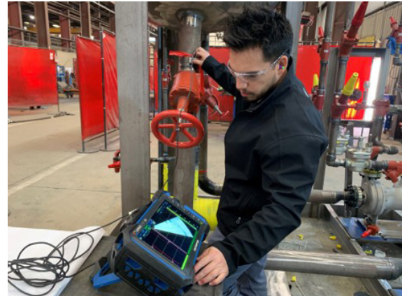
Figure 4: Phased Array Ultrasonic Testing.
