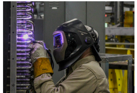
Figure 2: Welding return bends on a coil.
