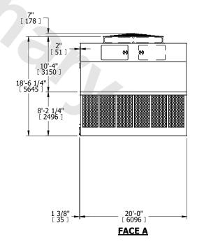
DRAWN BY: KDS NO. OF SHIPPING SECTIONS **SHIPPING** OPERATING HEAVIEST SECTION 6620 lbs+ [3005] kg+ 4200 lbs+ [1910] kg+ 11580 lbs+ [5255] kg+ WEIGHT WEIGHT WEIGHT
