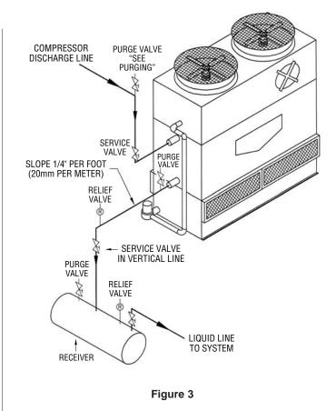
This allows the pressure in the receiver to be equalized with the pressure at the coil outlet and thus will allow free liquid flow from the condenser outlet to the receiver. The liquid drain line should also be pitched at least 1/4 inch per foot (20mm per meter) toward the receiver to facilitate this flow.
