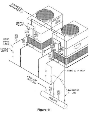
An alternative method for trapping liquid outlets on multiple condenser installations is illustrated in Figure 11. All the outlets are piped together into one liquid header. A single inverted "P" trap in used to create a liquid seal on the entire header. In order to prevent the refrigerant from siphoning from the <u>header</u>, the equalizer line must connect into the top of the inverted trap as a vacuum breaker as shown in close-up in Figure 12.
