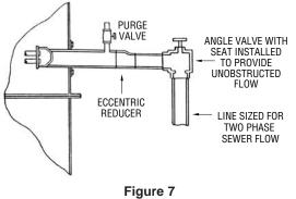
In this arrangement the drain line should always be sized for two phase sewer flow regardless of the hookup. It is recommended, for best results, that the velocity be kept as low as possible, particularly if an angle valve is installed.
