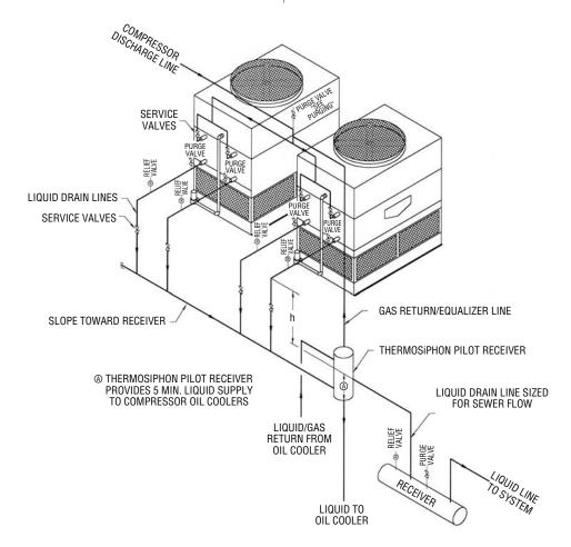
receiver then feeds liquid refrigerant to the oil coolers by gravity. In the oil coolers a part of the liquid is converted to vapor in the process of cooling the oil. The liquid-gas refrigerant mixture is returned to the pilot receiver and the vapor generated is separated in the receiver and returned to the condenser through the gas return/equalizer line. The rest of the liquid refrigerant flows from the pilot receiver to the main receiver and then on to the rest of the system.
