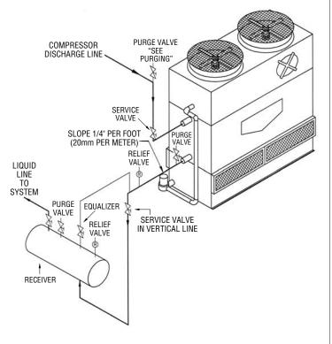
Evaporative condensers are often provided with oversized outlet connections. In this case the drain line can be reduced from the size furnished by the factory and still meet the criteria. It is permissible to reduce the line as shown in Figure 6, but it is recommended that it be done in the vertical portion of the line. If using this method, then the installation of shut off or service valves is preferred in the vertical portion of the line, and at least a foot below the horizontal portion.
