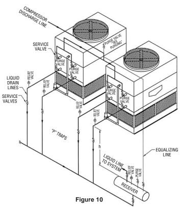
Again, the most important aspect of multiple unit hookups is the condenser to receiver liquid drain line piping. The key is to *trap it!* The drain line from each coil outlet must have a trap in the vertical portion of the line. This can be accomplished with a small "P" trap as illustrated in Figure 9 or by using a bottom inlet receiver as illustrated in Figure 10.
