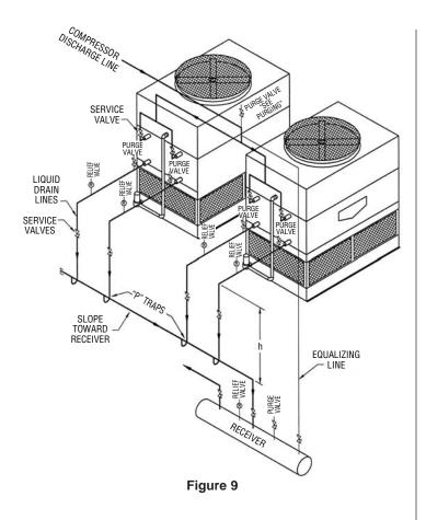
Figure 9 illustrates two large condensers piped in parallel to a single high pressure receiver. Note that the compressor discharge line should be piped as symetrically as possible. The earlier comments in regard to the sizing of these lines also apply to multiple condenser installations.
