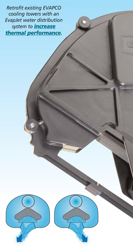
The fluidic geometry of the EvapJet nozzle breaks the fluid into two separate paths. Typically when the two fluids meet head on they will create a planar water stream however, the EvapJet nozzle is designed such that the streams meet at an angled approach. This design results in an oscillatory motion characteristic of fluidic nozzles.
