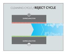
Supercapacitors reverse polarity to reject ions to drain at reduced flow rate
