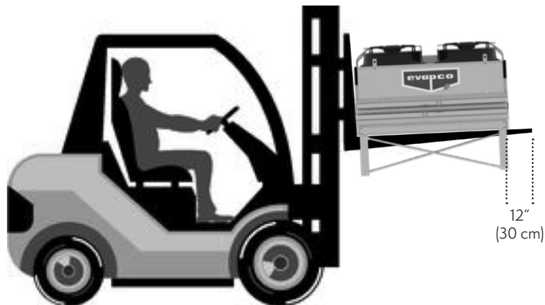
Figure 4 – Flat Coil Units Forklift Lifting Requirements
