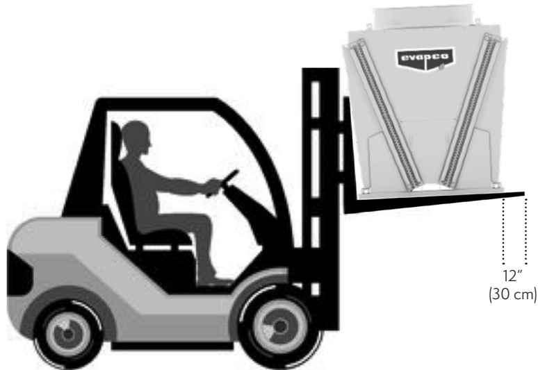
Figure 12 – V Coil Unit Forklift Lifting Requirements
