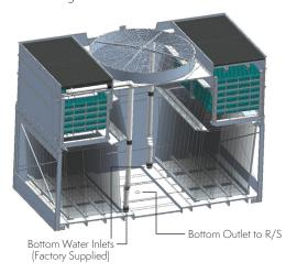
Note: When individual supply lines are piped to the PHC condenser balancing valves are recommended to ensure equal flow to each side of the condenser water distribution system.
