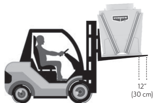
Figure 12 – V-Coil Unit Forklift Lifting Requirements
