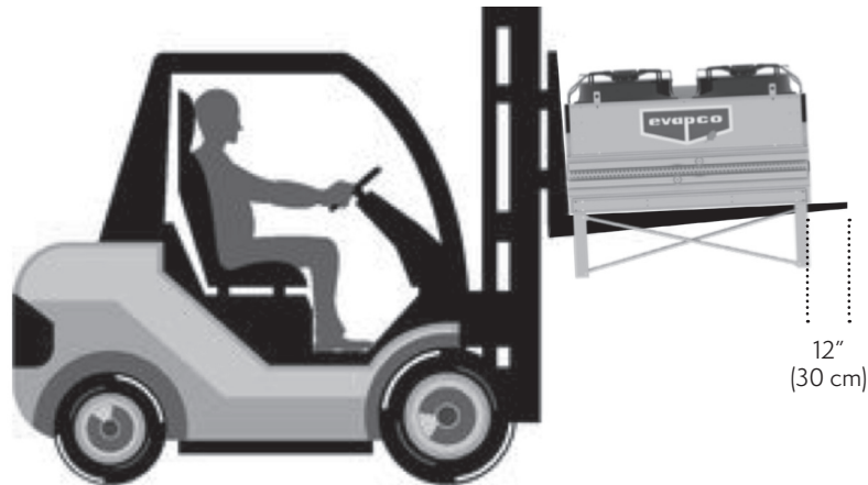
Figure 4 – Flat Coil Unit Forklift Lifting Requirements
