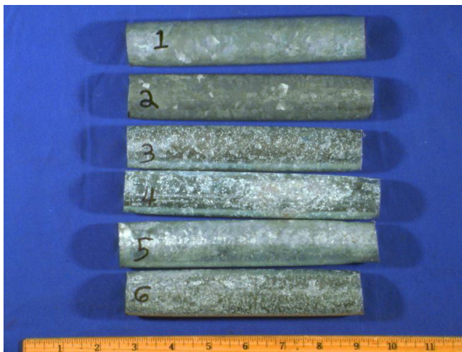
Figure 2: Galvanized Coil Samples From Tiny Coolers (SEM-EDXA)
