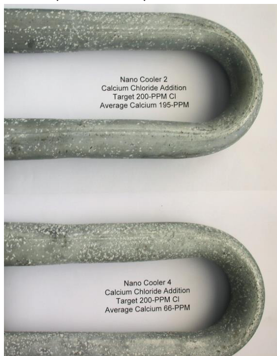
Figure 9: Higher Calcium (Nano Cooler 2) vs. Lower Calcium (Nano Cooler 4) Coil Sections
